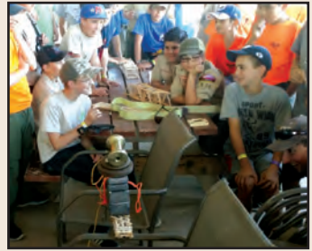
The addition of weights to Popsicle bridges determined the winning Scout team. The winning “flat bridge design” withstood 75 pounds before collapsing. Photo by Doug Wright.
