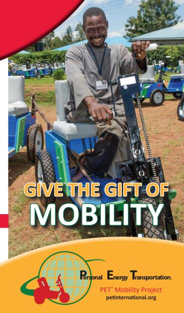
PET is a three-wheeled, off-road wheelchair, operated by hand power.
